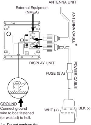
\* = Do not confuse the antenna cable with the transducer cable for the Echo Sounder (ex. LS-6100). The transducer cable is black; the antenna cable is white and "RADAR" is written on the cable.
