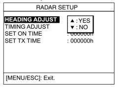
Radar setup menu (heading adjust)
