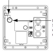
Make a hole of \$16. Seal hole with sealing compound after connecting cable.
