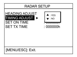
Radar setup menu (timing adjust)
