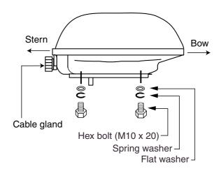
Antenna unit, showing location of mounting hardware
